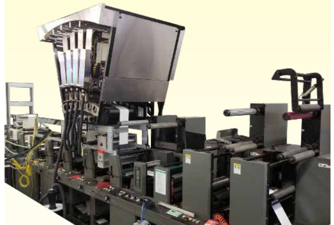
DICEweb retrofit on to a flexo press
